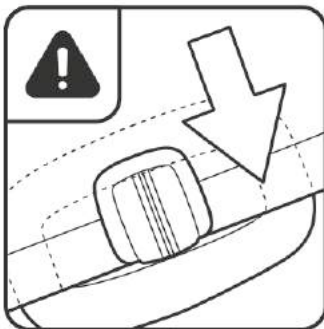
Figure 7: Symbol on packaging to indicate that the snap should be positioned downwards
